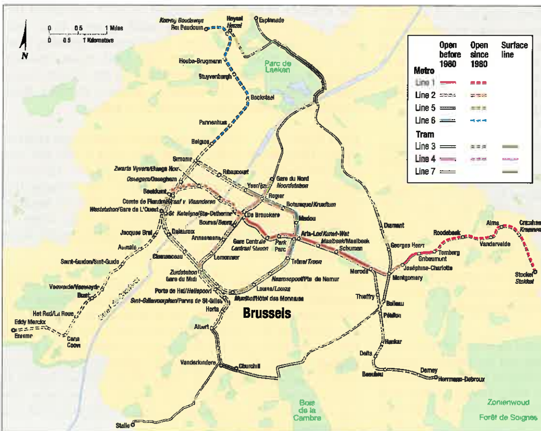
FIGURE 13-39 BRUSSELS, BELGIUM, METRO AND TRAM European cities such as Brussels have invested substantially in improving public transportation in recent years. Brussels provides a good example of a public transport system that integrates heavy rail (Métro) with light rail (trams). Trams initially used Métro tunnels, but the tunnels were large enough to convert to heavy-rail lines as funds became available.
